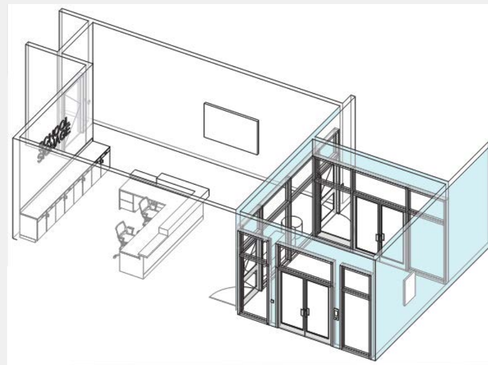
CISD Design Guidelines - Typical Secure Vestibule Upgrade
