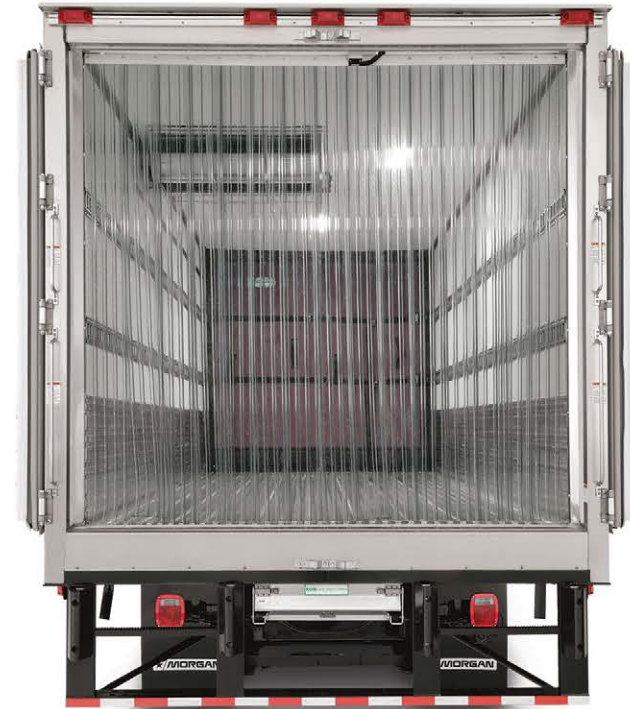
Cargo Interior Shown With E-track, Bulkhead/Multi-Temp Configuration and Strip-Curtain
