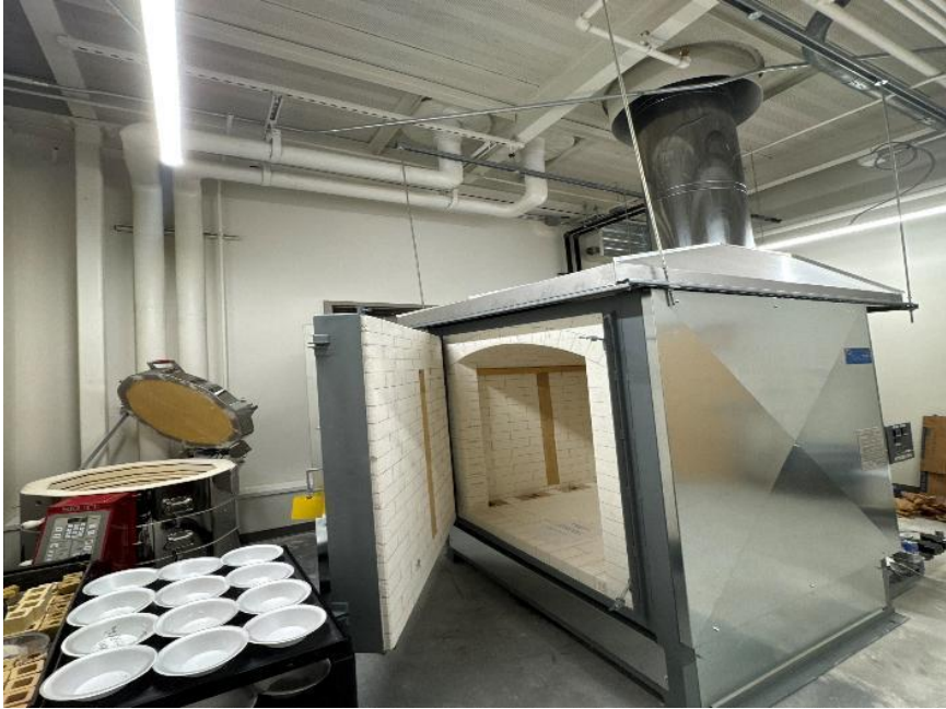
Geil Kiln set in place and ready to be connected
