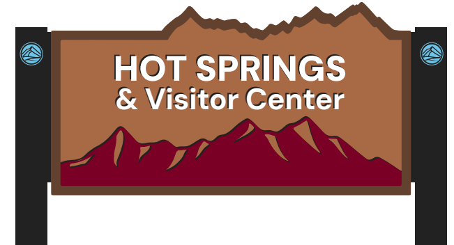
LOGO PLACEMENTS ON STEEL BEAMS BLUE OR WHITE LOGOS BLACK POWDER COATED STEEL BEAMS
