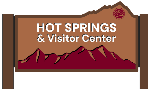
MINIMIZED MOUNTAIN LANDSCAPE AT TOP TOP RIGHT MAROON OR WHITE LOGO BROWN POWDER COATED STEEL BEAMS
