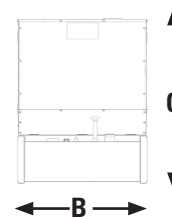
Sound Attenuated Enclosure on a UL Listed Integral Fuel Tank Base
