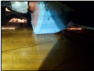
Dirty friction drive rollers.
