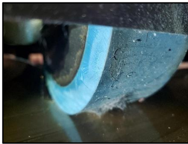
Dirty friction drive rollers.
