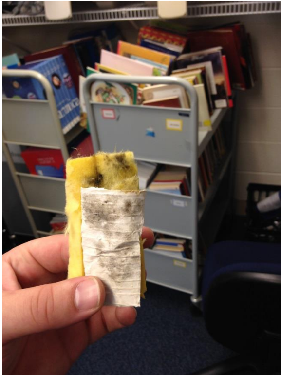
Photo 51 – Bulk sample collected from Library storage confirmed as containing mold growth
