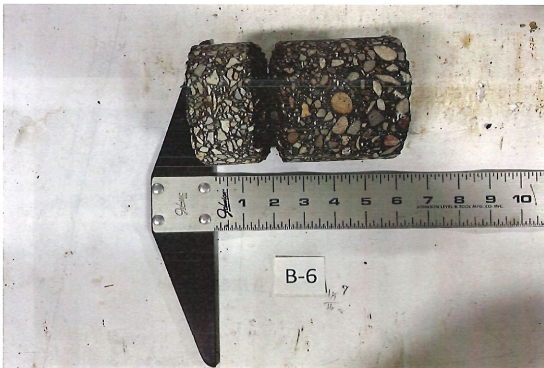
Pavement Core B-6: Spaulding Elementary School
