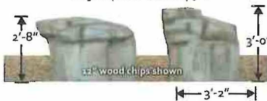
12" of woodchips -or- EPDM surfacing and fill. 12" of part must be installed below top of surfacing.
