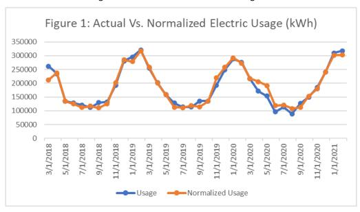
Normalizing the actual usage against days in billing cycle, heating degree days (base 65), and cooling degree days (base 65) resulted in an  $R^2$  = 0.99, which suggest there is a strong relationship between electric usage in the dependent variables. Baseline electric usage can be defined by the following formula:
