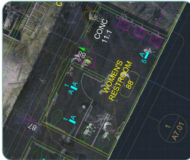
Example 3D scan overlaid with proposed draws to identify any potential conflicts with existing conditions.
