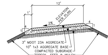
**GRAVEL DRIVE CROSS SECTION A-A**
