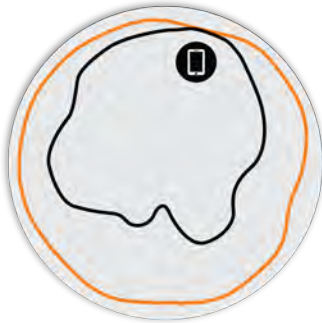
Figure 2. R650 2.4GHz Azimuth Antenna Patterns
