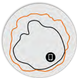
Figure 6. R670 5GHz Elevation Antenna Patterns
