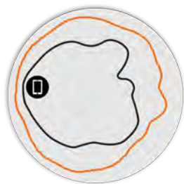
Figure 5. R670 2.4GHz Elevation Antenna Patterns
