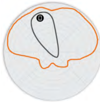
Figure 4. T750 2.4GHz Elevation Antenna Patterns
