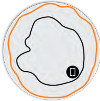
Figure 3. R650 5GHz Azimuth Antenna Patterns
