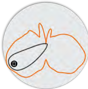
Figure 6. R560 5GHz Elevation Antenna Pattern
