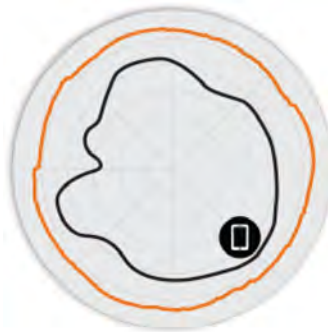
Figure 3. T750 5GHz Azimuth Antenna Patterns
