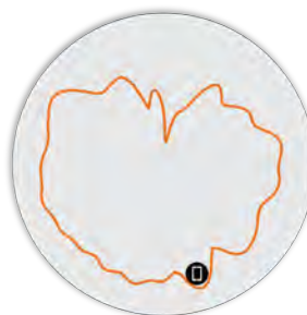
Figure 6. R560 5GHz Elevation Antenna Pattern
