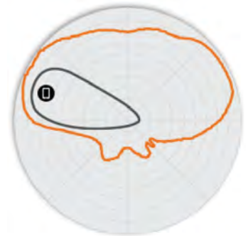
Figure 5. T750 5GHz Elevation Antenna Patterns
