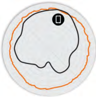
Figure 2. T750 2.4GHz Azimuth Antenna Patterns
