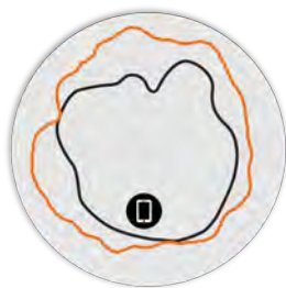
Figure 7. R670 6GHz Elevation Antenna Patterns
