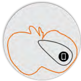
Figure 5. R670 2.4GHz Elevation Antenna Patterns
