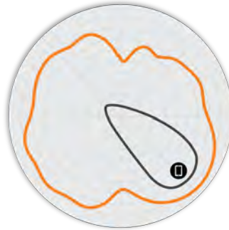
Figure 4. R650 2.4GHz Elevation Antenna Patterns
