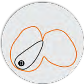
Figure 5. R560 2.4GHz Elevation Antenna Pattern
