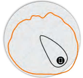
Figure 5. R650 5GHz Elevation Antenna Patterns
