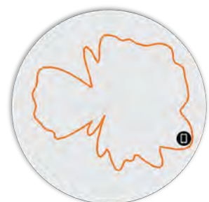
Figure 7. R560 6GHz Elevation Antenna Pattern
