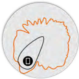
Figure 6. R670 5GHz Elevation Antenna Patterns
