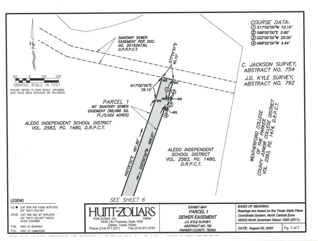
Correct Ending Coordinates, North: 0.000 East: 0.000 Ending Coordinates, North: 0.008 East: 0.004 Error, N: 0.01 E: 0.00 Total: 0.01 Brg: S 26°43'21"W Distance Traversed: 4496.38 Closure: 489080
