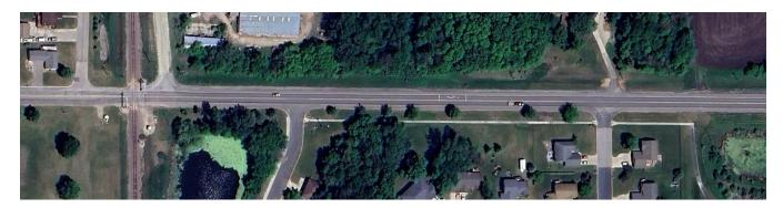
East of 6<sup>th</sup> St., out past the school entrances, the school bus garage, and to CSAH 1, it is our determination that no reduced speed limit is appropriate or warranted. That roadway segment is designed as a rural type roadway, with full shoulders, and can safely accommodate vehicles traveling at the statutory speed limit of 55 MPH.
