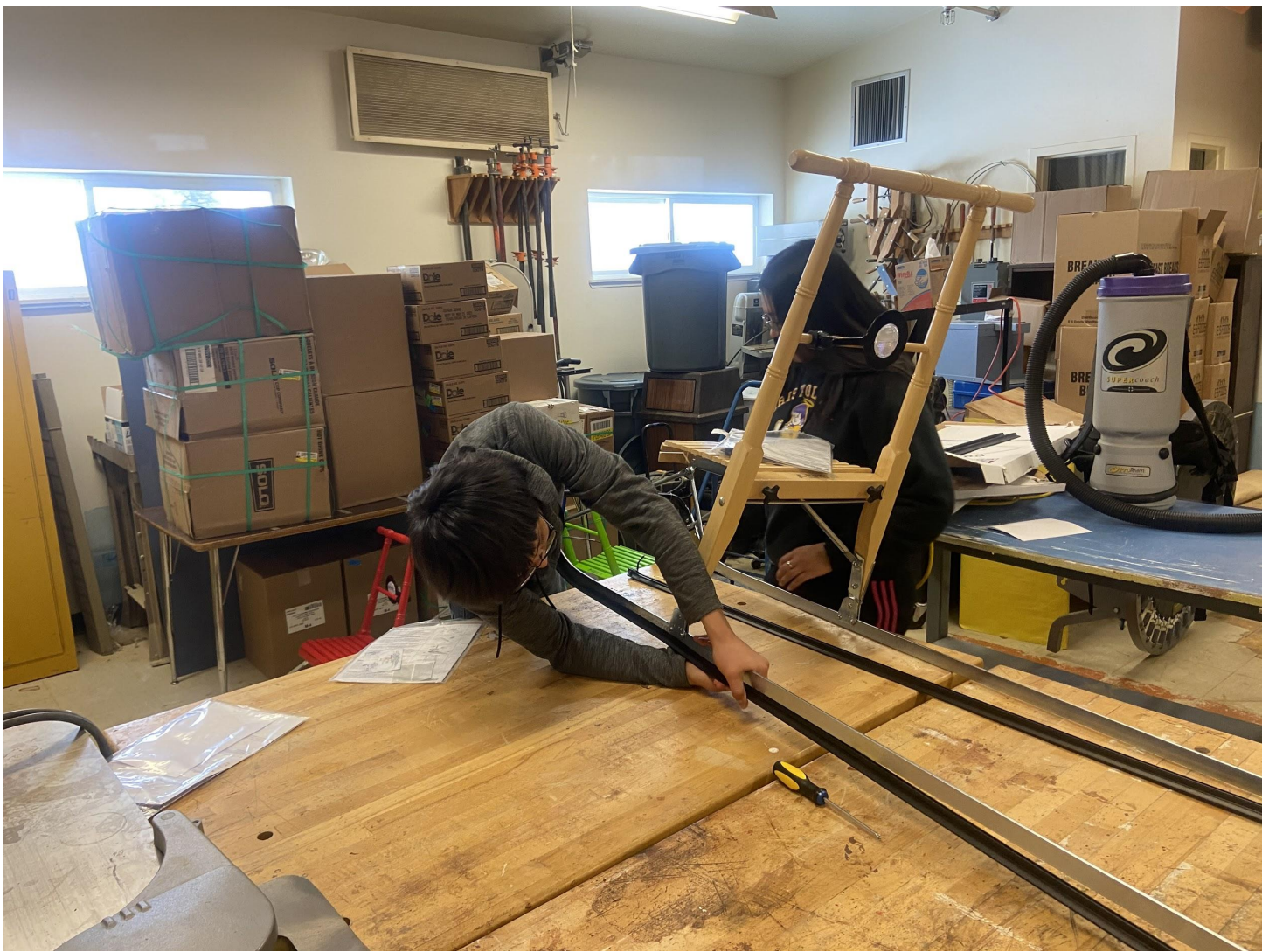
Members of the student government worked to assemble all of the kicksleds that were purchased. Here John (8th) and Nyssa (11th) Tallekpalek team up to attach runners to a kicksled.
