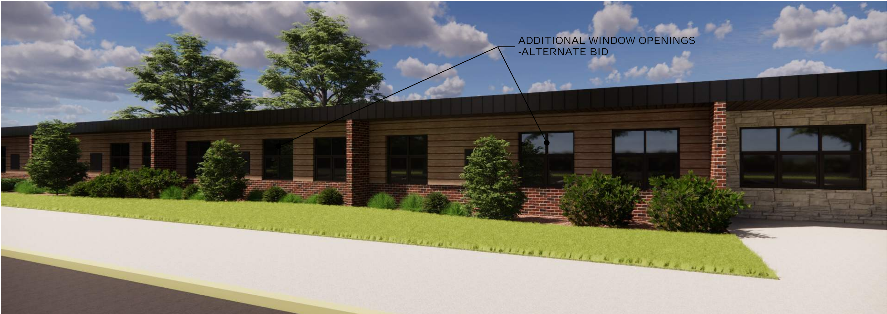
NEW PANELING REPLACES OLD PANELING ON SCHOOL ELEVATION, NEW WINDOW TYPE, AND NEW WINDOW FENESTRATION
