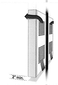
DO NOT RESTRICT AIRFLOW on the cabinet's rear side. A minimum 2" gap per face behind each cabinet is necessary. For wall-mounted rear-vent cabinets, airflow must be unobstructed from top to bottom, in addition to leaving a minimum 3" gap between the sign and wall.
