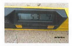
8. Nowhere shall the cross slope of an accessible route exceed 1:50 [cross slope of the route leading to the ramp = 5.3%]. IAC § 400.310(a)(6).
