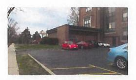
2. The surface slope of the accessible parking space's vehicle space exceeds 1:50 or 2% [2.7% (middle cross), 2.6% (bottom cross)]. IAC § 400.310(c)(3).
