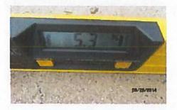
9. The running slope of an accessible route/walking surface shall not be steeper than 1:20 [running slopes range from 6.7% - 10.0%]. IAC § 400.310(a)(6); Standards § 403.3.
