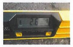
3. The surface slope of the accessible parking space's access aisle exceeds 1:50 or 2% in all directions [2.1% (top running slope), 3.9% (top cross slope) and 2.1% (bottom cross slope)]. IAC § 400.310(c)(3).
