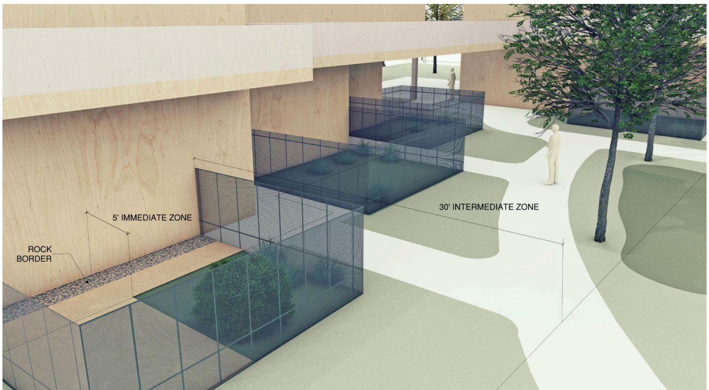
Above: Firewise zones example on site, based on CEAP wildfire planning guidance and Firewise USA best practices
