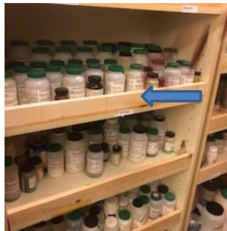
Installed toe boards on chemical shelving
