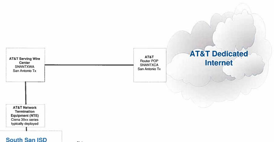
7535 Barlite Blvd 1Gbps ADI service AT&T provided and maintained router. AT&T typically provides Cisco ASR series router
