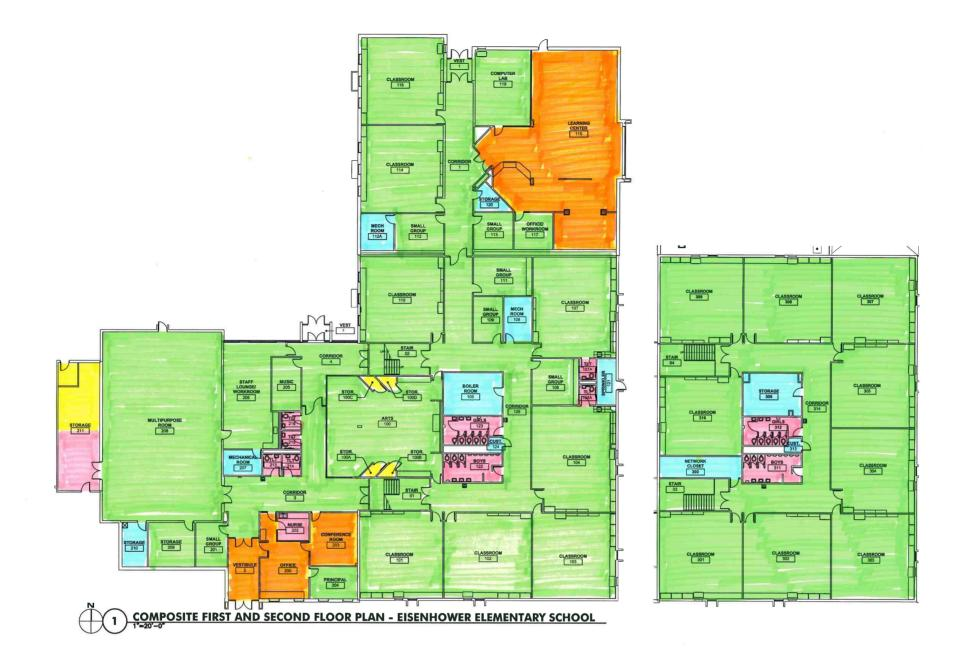
This color coded example of IKE shows specific building areas assigned by APPA service levels. Level 1 receiving the most detailed, labor intensive service, 5 the least.
