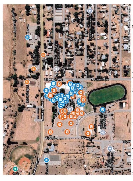
New and existing cameras. New cameras are blue, existing cameras are orange. Their existing NVR and software system is Genetec.
