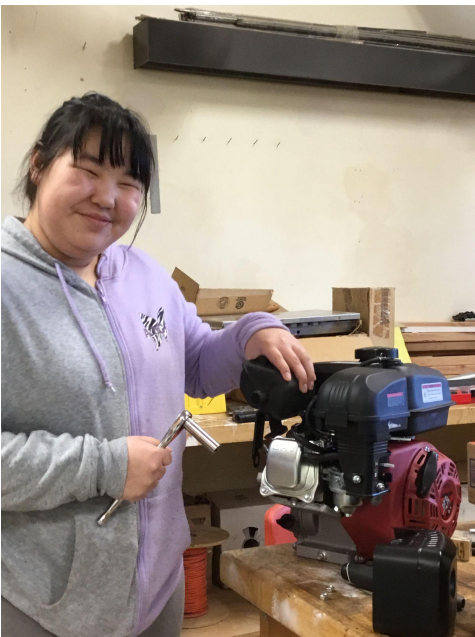
Maddy Apokedak removes the exhaust from an engine.
