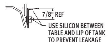
Sectional View Showing Table Connections
