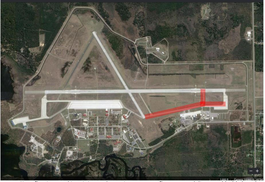
Fix reflective cracking, joint seal, repair pavement flaws, remark lines and hold short bars
