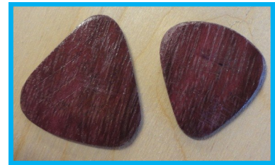
Guitar picks made by BillyW in Manufacturing Technology class using purple heart wood.
