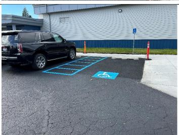
ADA access aisle to be 8' wide minimum. Provide additional ADA VAN stall and ADA signage.
