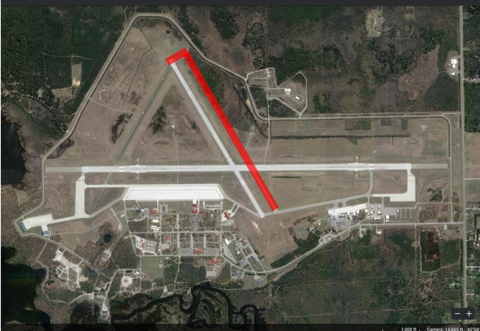
This will create a full-length taxiway to prevent back taxiing on an active runway
