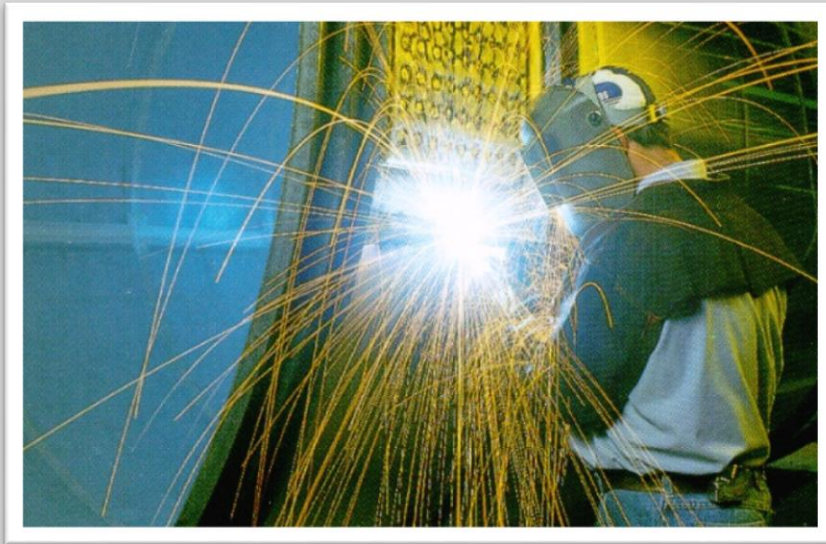
Welder at DCI, Inc. welding a heat transfer jacket on a vessel.
