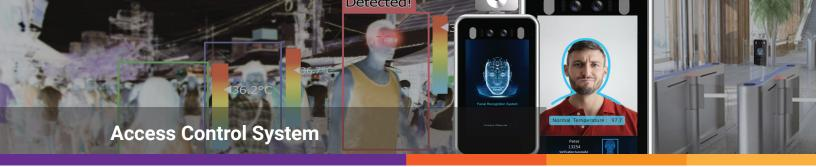
The ANT Q9 is an Access Control System that individually measures the body temperature of employees entering facilities. This Smart Access Control terminal combines infrared temperature measurement with 3-in-1 facial recognition. Intelligent analysis has mask detection capabilities and records date, time, body temperature and other details.
